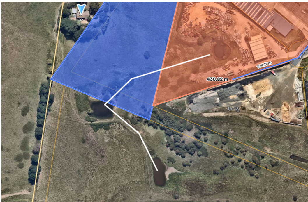
Figure 4.3: Pre-development flow path for southern hydroline (Nearmap)
